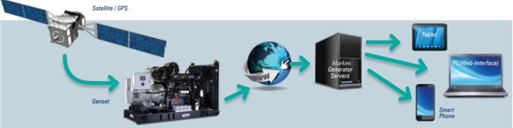
Markim Remote Monitoring and Management System, supported by GSM and internet technologies, is a highly useful and costeffective web-based solution that allows remote generator monitoring and intervention when needed. This system, which has the latest technologies, sends the working data of the generator on the field via the control panel to a remote device such as a computer, tablet or smartphone and allows the generator to be managed via this device.
